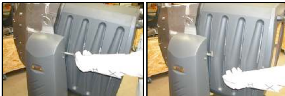
Locking the tilt axis
