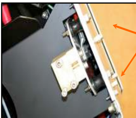
Shock absorbers mounted cathode support of the Osram 4.5Kw lamp
