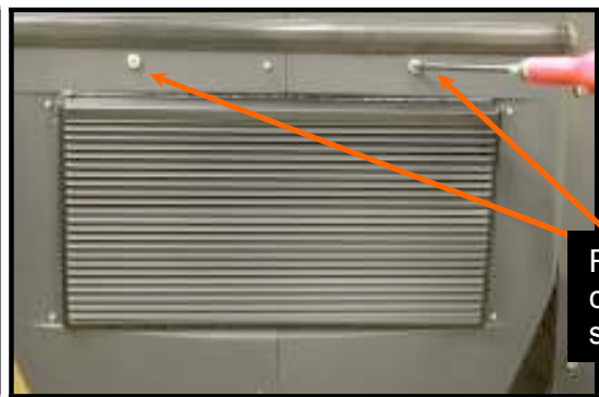
Rear cover fasteners
